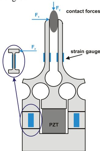
Fig. 3. Modified micro-gripper with force sensing
