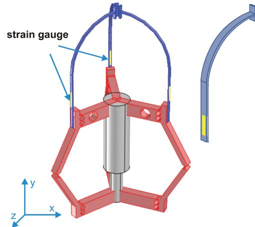
Fig. 5. RCC gripper with force sensing
