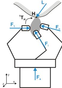
Fig. 1. Grasped object with contact forces
