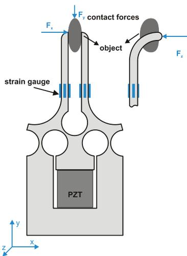
Fig. 4. Modified micro-gripper with force sensing – bending of micro-gripper fingers
